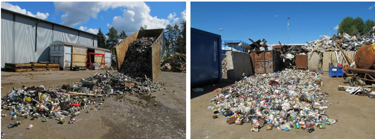
Figure 4. Spreading of loads for sampling.
