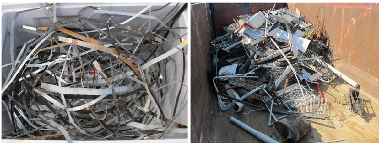
Figure 5. Larger metal pieces removed from the loads before sampling. Left: packaging metal, right: small metal items.
