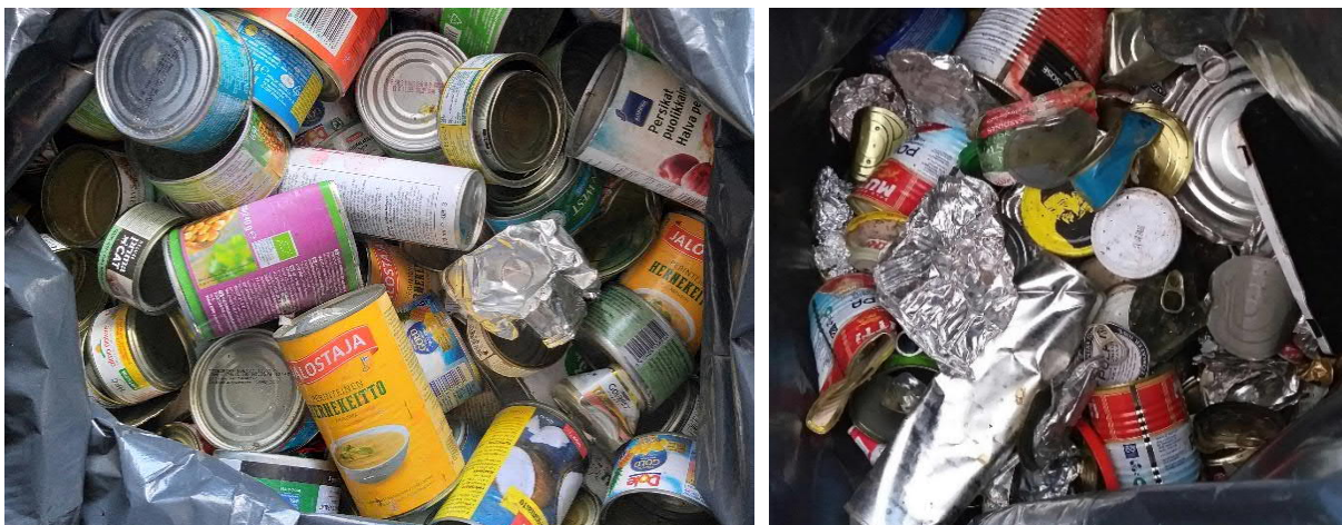
Figure 17. Metal Packages, left the dirty fraction and on the right clean fraction.
